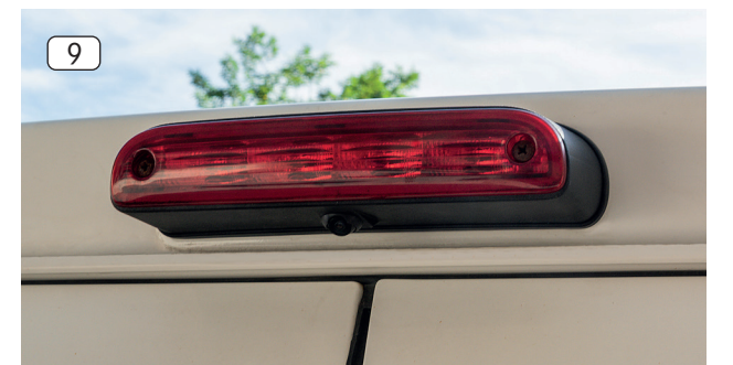
9. Alignment of the camera ball at the bottom side of the camera main body if necessary, using the supplied U-shaped tool.
