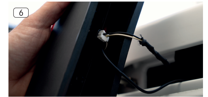
6. Connect the system plug with the connector counterpart of the brake light reflector housing.
