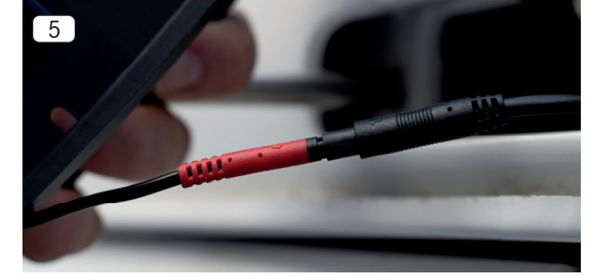
5. Connect the 4PIN mini connector of the camera sensor to the mini connector counterpart of the main wire. Wrap around some isolating tape to secure the connectors.
