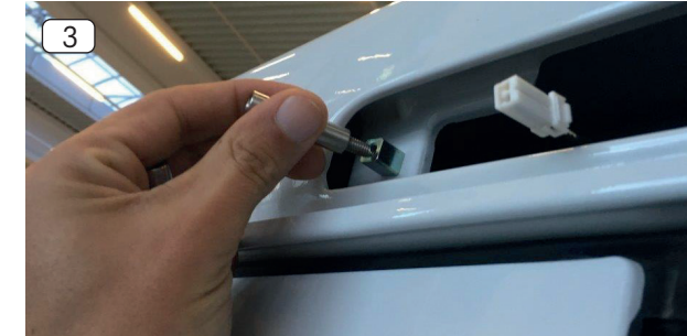
3. Screw in and tighten the stainless steel mounting bolts by hand (5Nm). Use a dab of Loctite, if possible.
