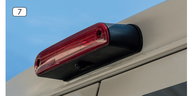
7. Re-mount the brake light reflector housing on top of the main camera housing, using the original Philips cross-recess screws.
